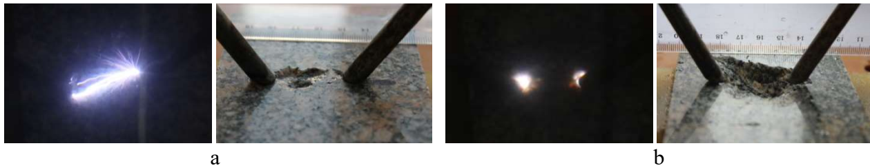
Fig. 5. Electrohydraulic (a) and electro-pulse (b) effects and results of their action on granite surface.
