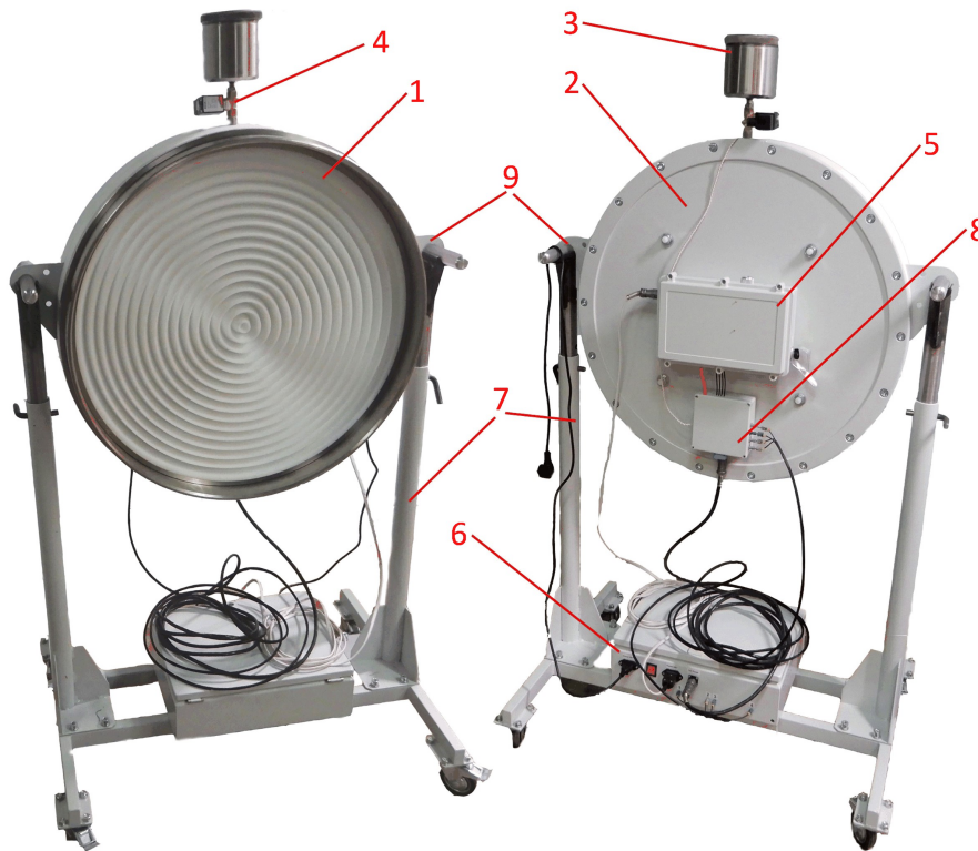
Fig. 2. Appearance of the calorimeter: 1 – absorbing load (front view), 2 – absorbing load (rear view), 3 – expander, 4 – top valve, 5 – control and registration unit, 6 – power supply, 7 – movable stand, 8 – block of electrical connectors, 9 – mounting brackets.
